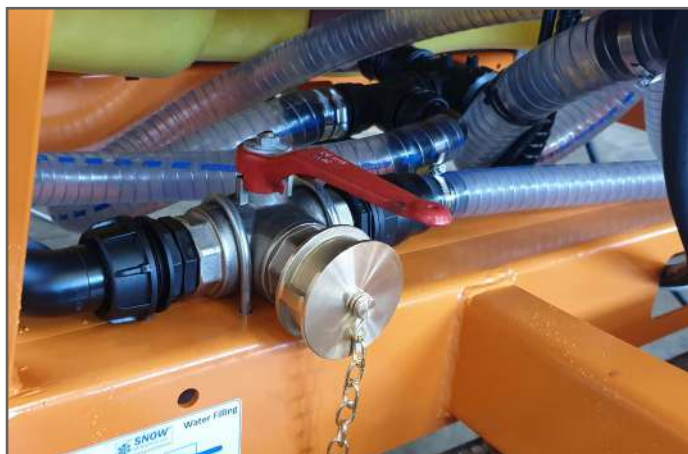
Manual valve with UNI-STORZ coupling for tank filling/emptying processes
