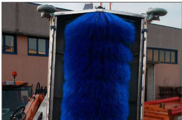
Cleaning brush (D 1000 mm, L 1800 mm)
