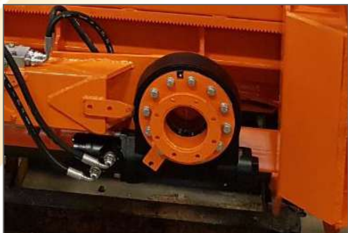
Hydraulic fifth wheel/circle frame for head rotation
